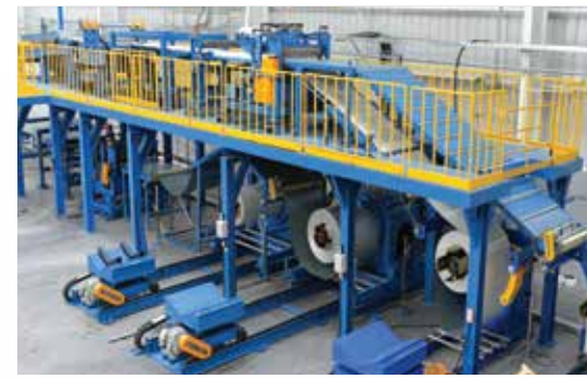
Uncoiler Mezzanine Deck
